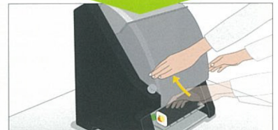
Press Start Switch right above the base.
