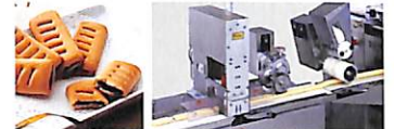
"Press Roller with Flour Duster" and "Blade Wheel" and "Vertical Cross Cutter"
